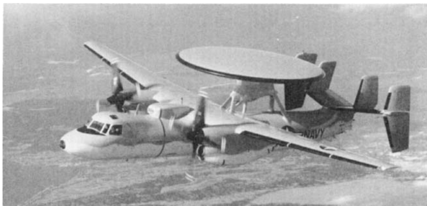
FIG. 16.1 E-2C airborne early-warning (AEW) aircraft showing rotodome housing the antenna.
