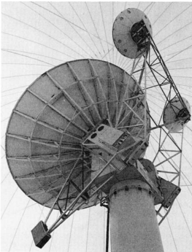
FIG. 23.6 The CP-2, multiple-parameter radar at the National Center for Atmospheric Research, Boulder, Colorado. (Courtesy of the National Center for Atmospheric Research.)
