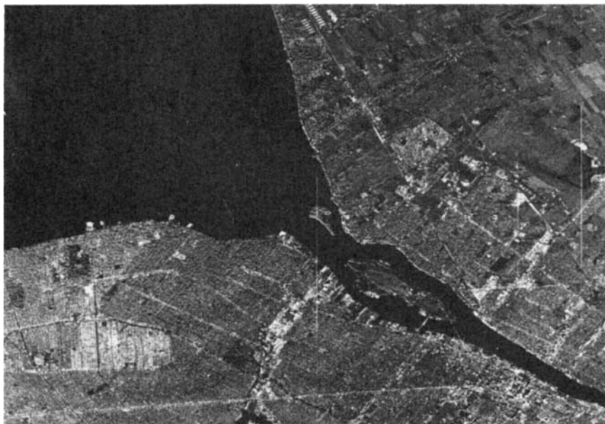
FIG. 21.5 STAR-1 radar imagery, lower Lake St. Clair, upper Detroit River. Resolution, 20 ft (6 m). (Courtesy Environmental Research Institute of Michigan.)
